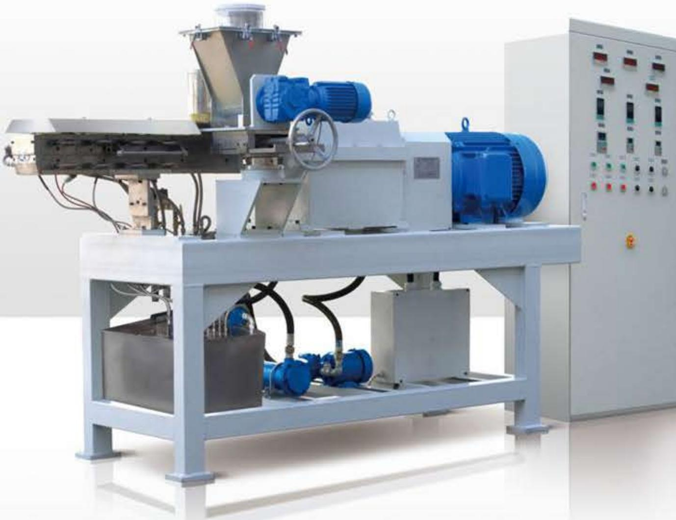
This series of extruder adopts co-rotating twin screw structure. Multi kinds of raw materials can achieve optimal dispersed and kneaded effect after fully hot-melted under the precise intermeshing action by the conveying elements and kneading elements mounted on the twin screws.
