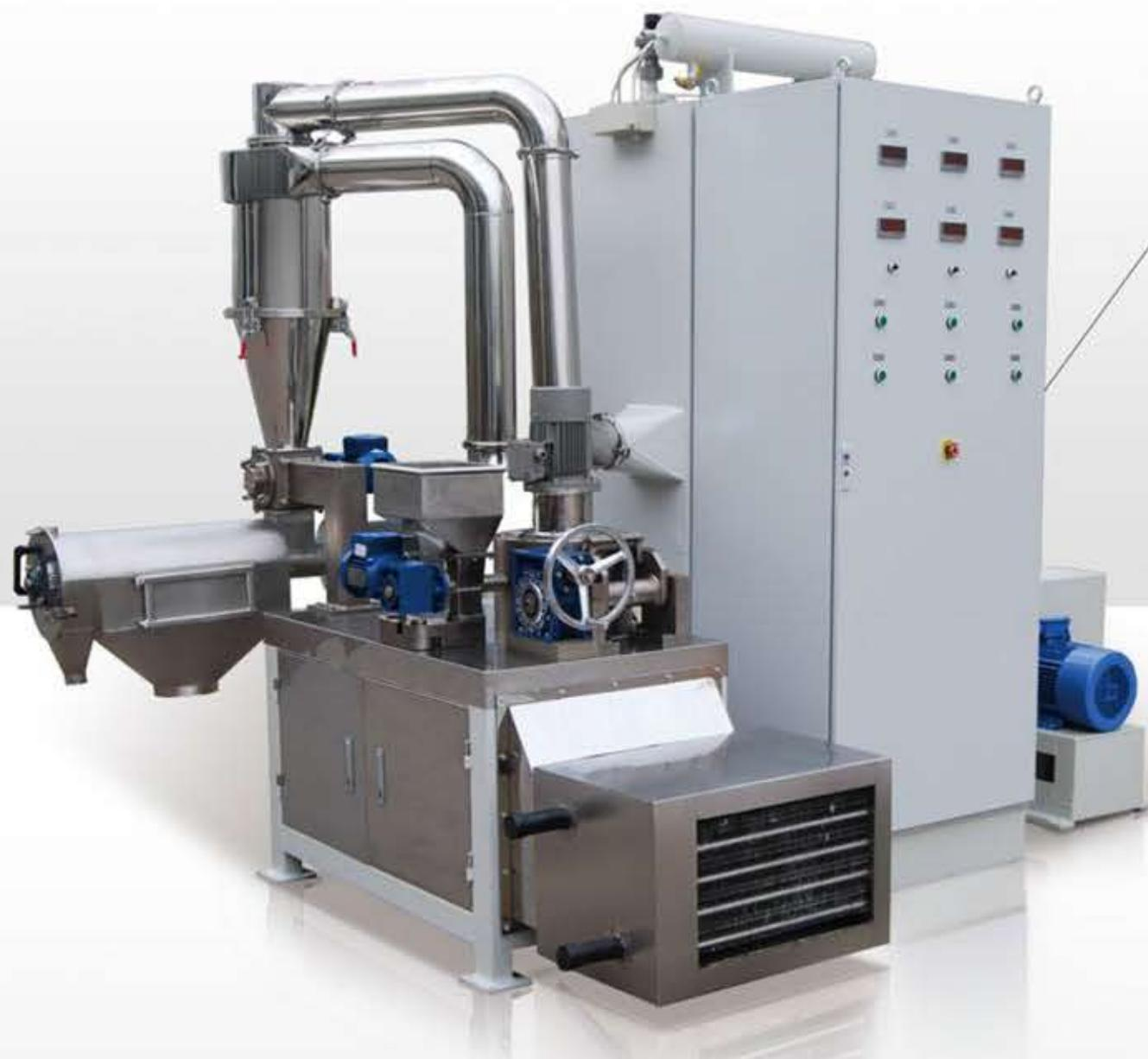
This series of grinding system is mainly used to make small sample and pilot sample in lab, in order to acquire the best formula and technical parameters in production. It adopts the newest technology in grinding craft, mechanical drive & structure, control system and etc.
